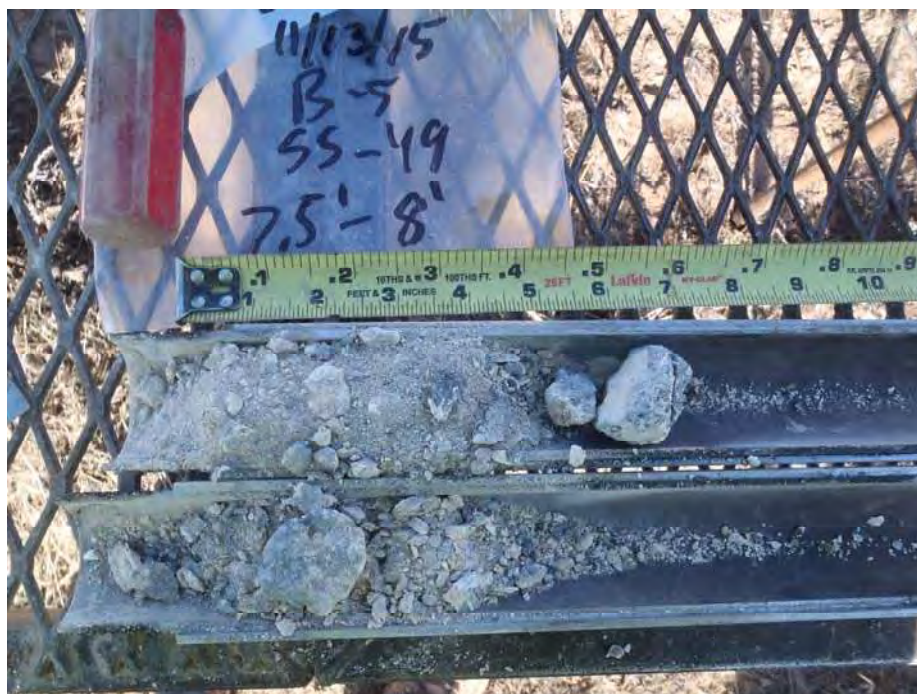
Photo 2: Boring B-5, sample SS-49 at 7.5 feet Poorly Graded Sand with Silt and Gravel (SP-SM)
