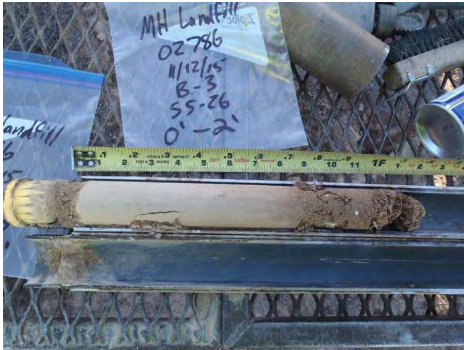
Photo 1: Boring B-3, sample SS-26 at 0.0 feet Sandy Silt (ML)
