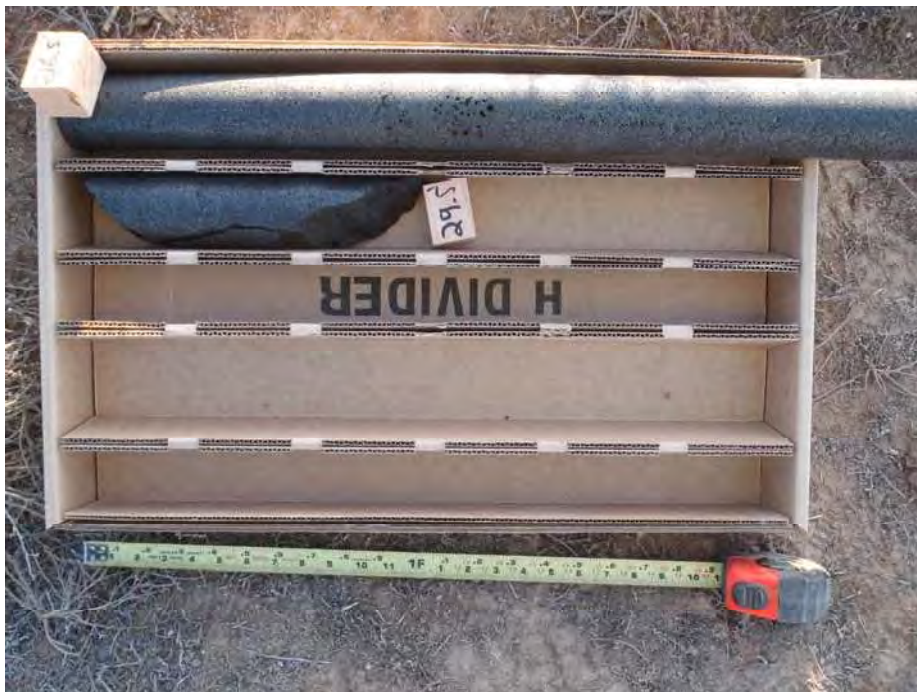
Photo 4: Boring B-3, Rock Coring from 26.5 to 29.5 feet Basalt Rock
