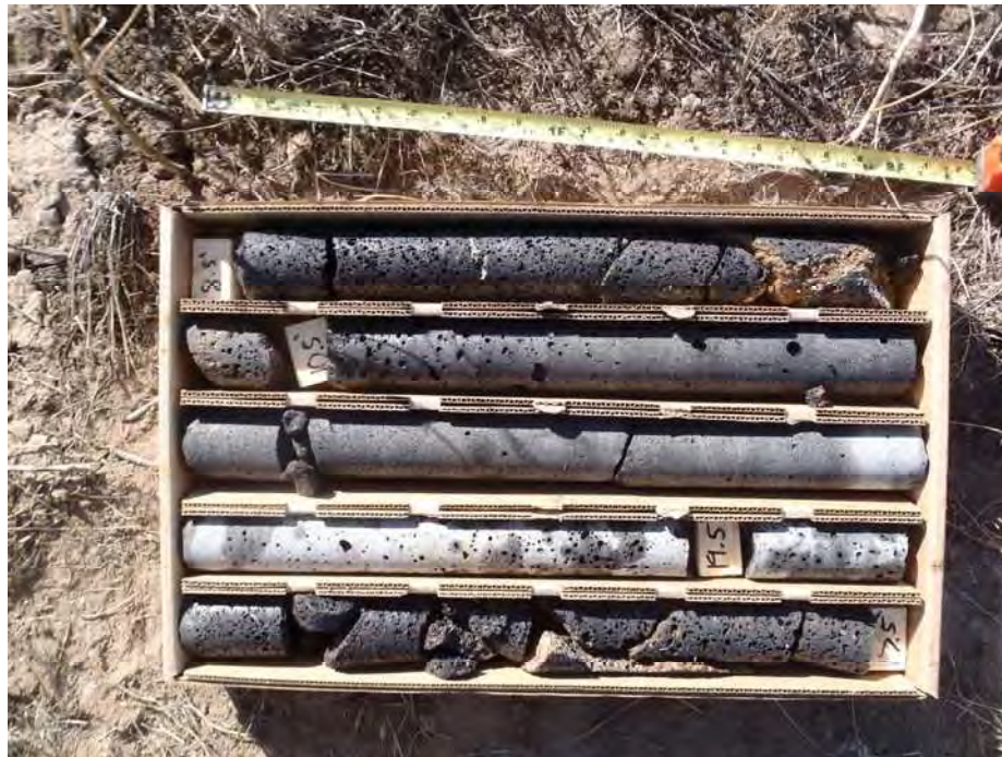
Photo 3: Boring B-5, Rock Coring from 8.5 to 17.5 feet Basalt Rock
