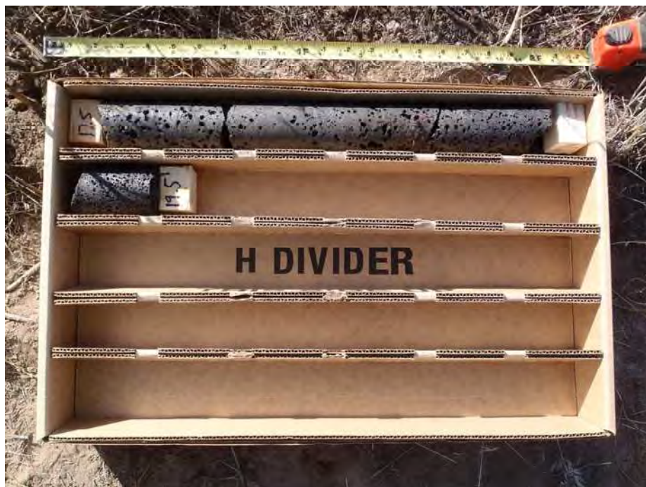
Photo 4: Boring B-5, Rock Coring from 17.5 to 19.5 feet Basalt Rock
