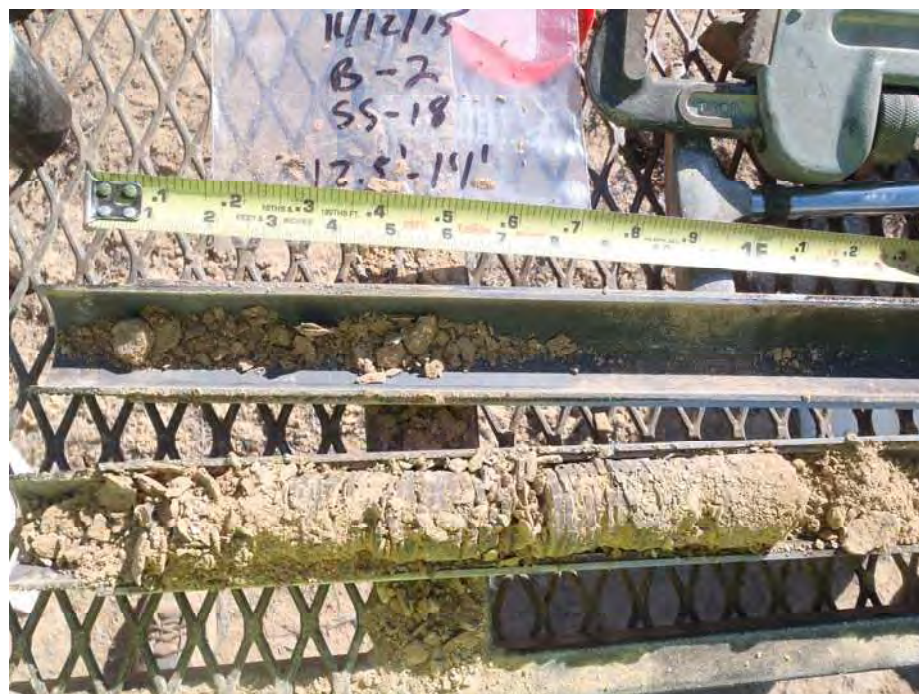
Photo 2: Boring B-2, sample SS-18 at 12.5 feet Sandy Silt (ML)
