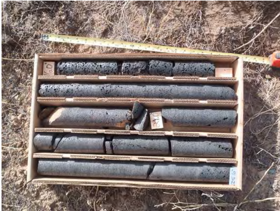
Photo 3: Boring B-4, Rock Coring from 16.0 to 26.0 feet Basalt Rock
