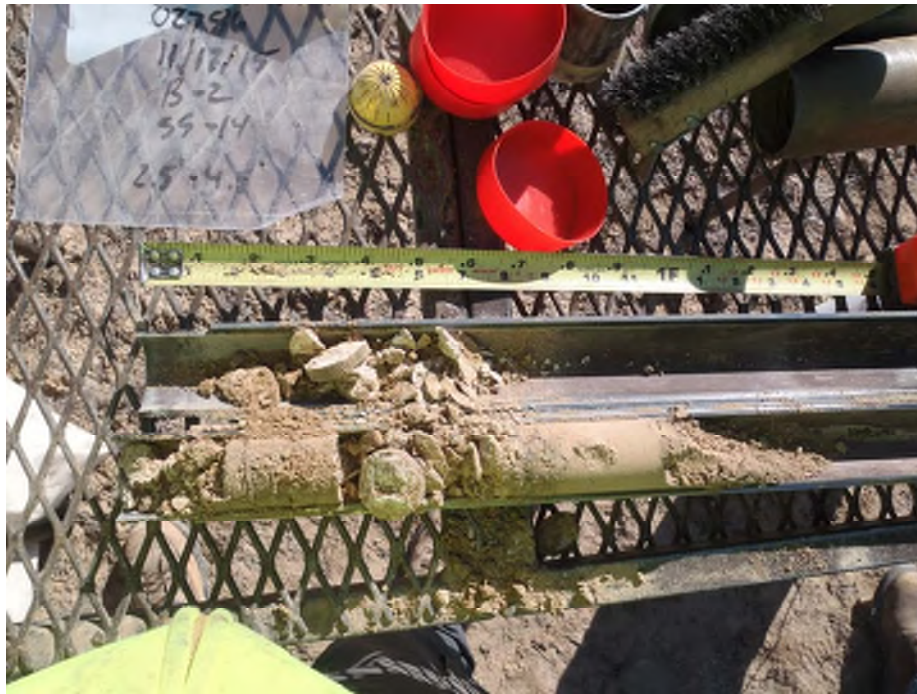
Photo 1: Boring B-2, sample SS-14 at 2.5 feet Sandy Silt (ML)
