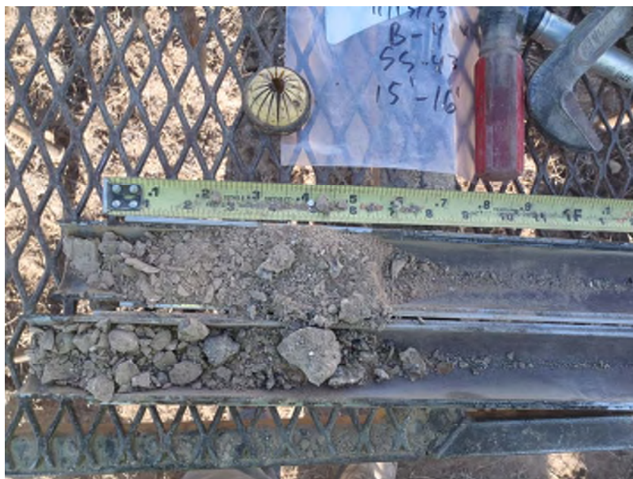
Photo 2: Boring B-4, sample SS-43 at 15.0 feet Sandy Silt (ML)
