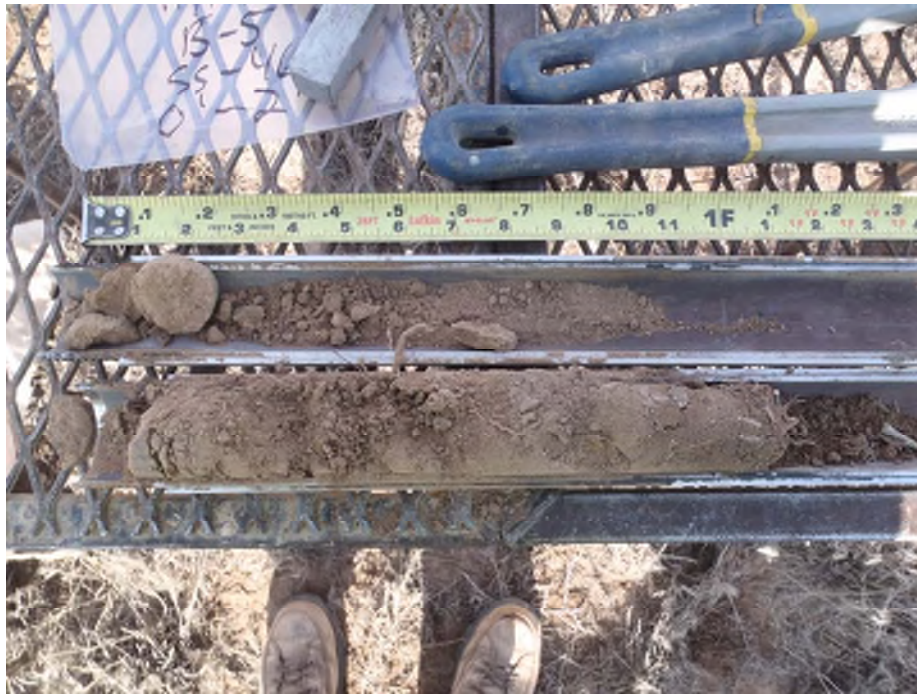
Photo 1: Boring B-5, sample SS-46 at 0.0 feet Sandy Silt (ML)
