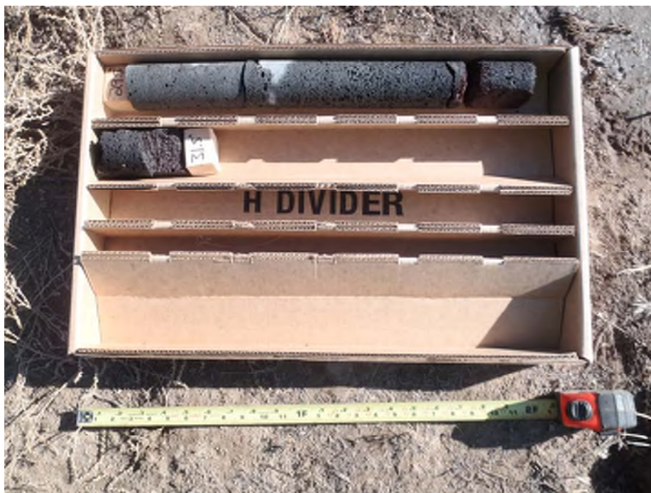
Photo 4: Boring B-1, Rock Coring from 29.5 to 31.5 feet Basalt Rock
