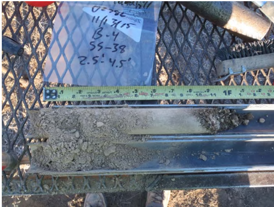
Photo 1: Boring B-4, sample SS-38 at 2.5 feet Sandy Silt (ML)
