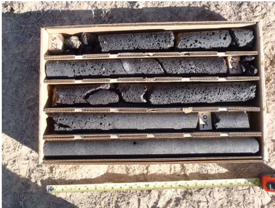
Photo 3: Boring B-2, Rock Coring from 22.5 to 33.3 feet Basalt Rock
