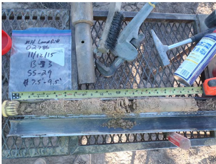
Photo 2: Boring B-3, sample SS-29 at 7.5 feet Sandy Silt (ML)
