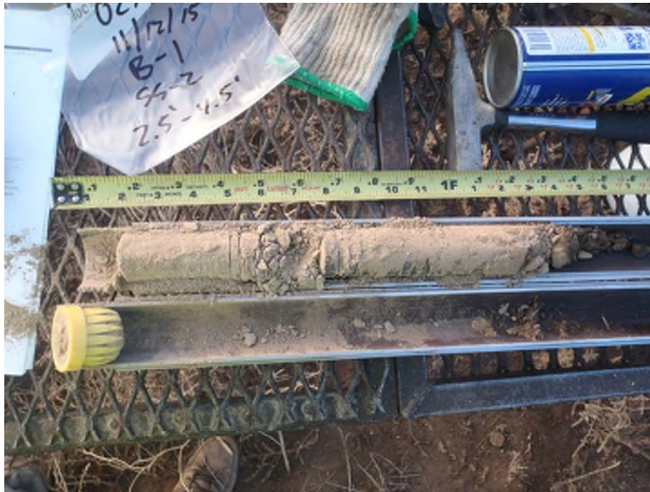
Photo 1: Boring B-1, sample SS-2 at 2.5 feet Sandy Silt (ML)
