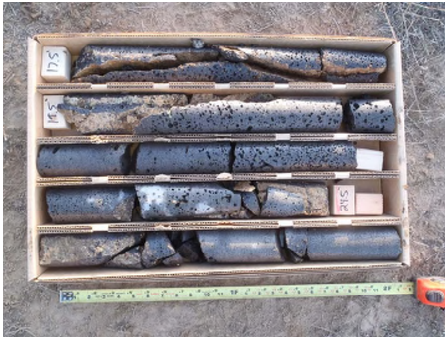
Photo 3: Boring B-3, Rock Coring from 17.5 to 26.5 feet Basalt Rock
