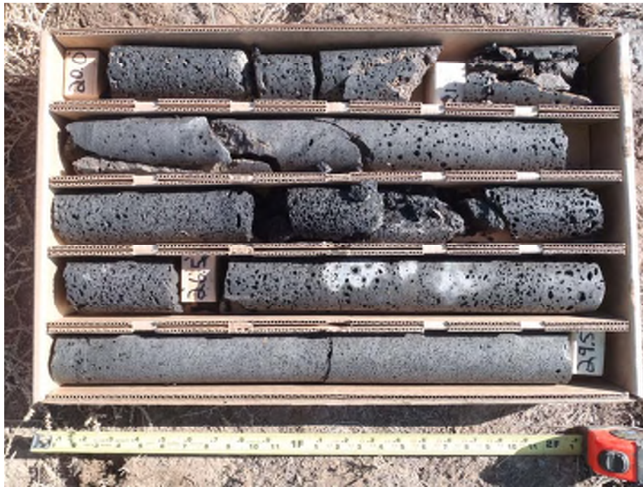
Photo 3: Boring B-1, Rock Coring from 20.0 to 29.5 feet Basalt Rock
