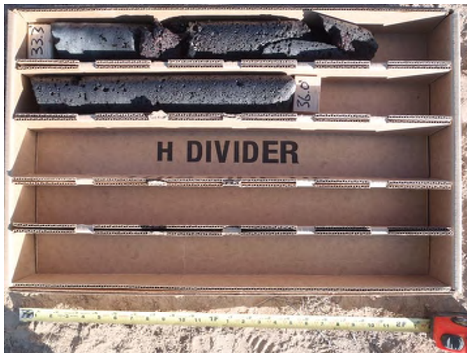
Photo 4: Boring B-2, Rock Coring from 33.3 to 36.0 feet Basalt Rock
