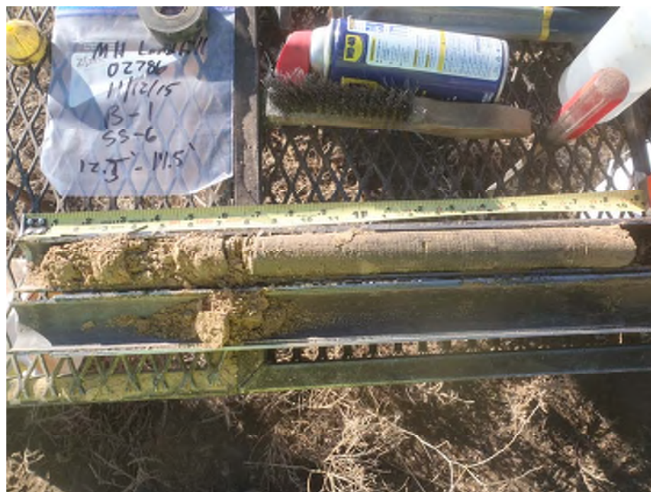
Photo 2: Boring B-1, sample SS-6 at 12.5 feet Sandy Silt (ML)
